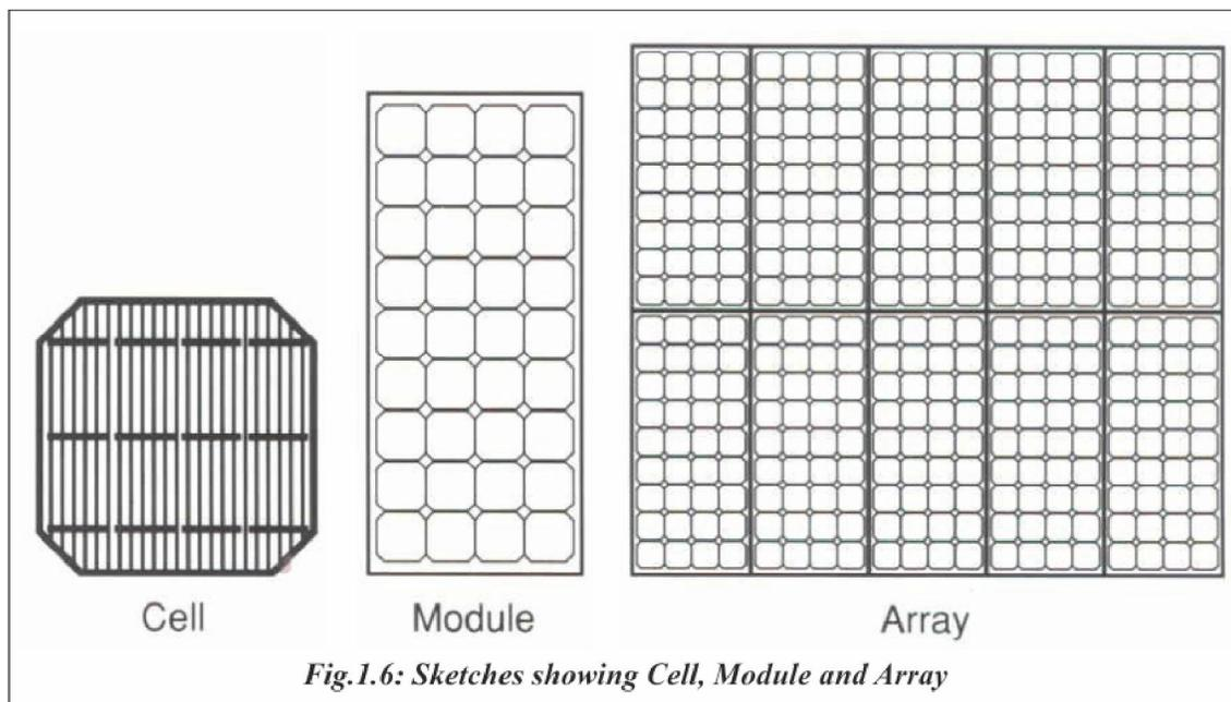
*Fig.1.6: Sketches showing Cell, Module and Array*
