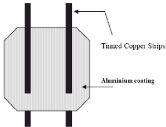
*Fig 1.2 (b) Sketch showing rear view of typical pseudo square solar cell*
