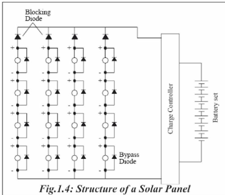
Fig.1.4: Structure of a Solar Panel
