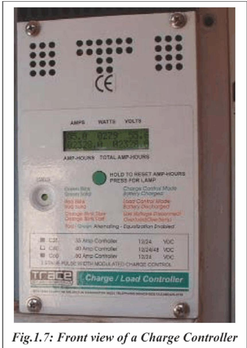
**Fig.1.7: Front view of a Charge Controller**
