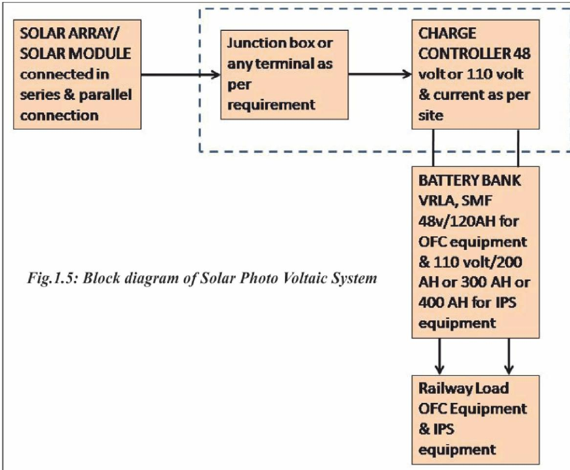
*Fig.1.5: Block diagram of Solar Photo Voltaic System*
